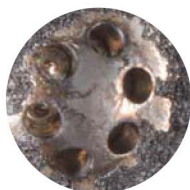
Injector after one P.i. treatment.
